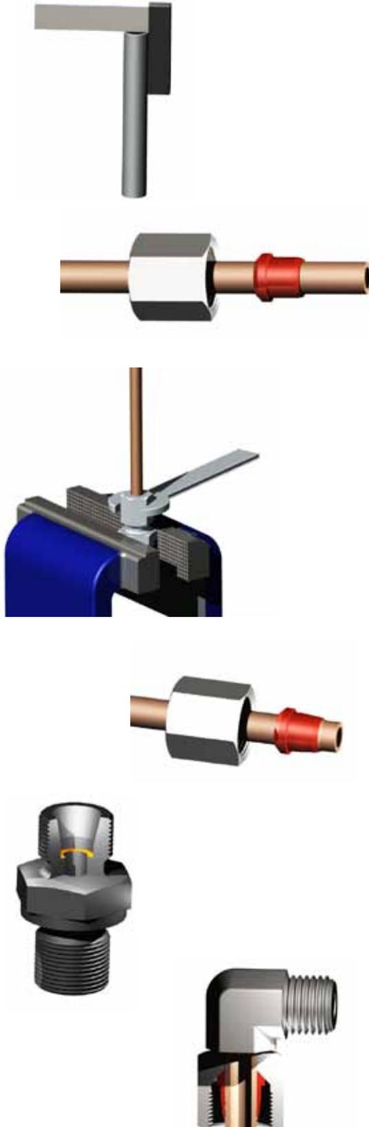
1. Cut the tube at a 90 degree angle (do not use roller, type tube cutters), remove all internal and external burrs.
